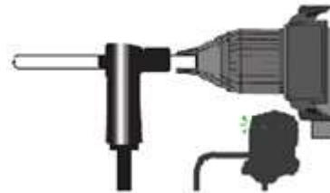
Hollow drill bit (Dustless drilling)
